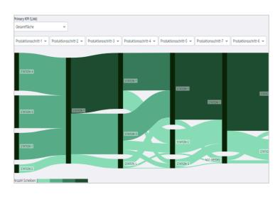
A Sankey diagram is used to visualise the material flow and the relationship between different work stations. Production can be analysed in a targeted manner by filtering for specific time periods, product or process attributes.
